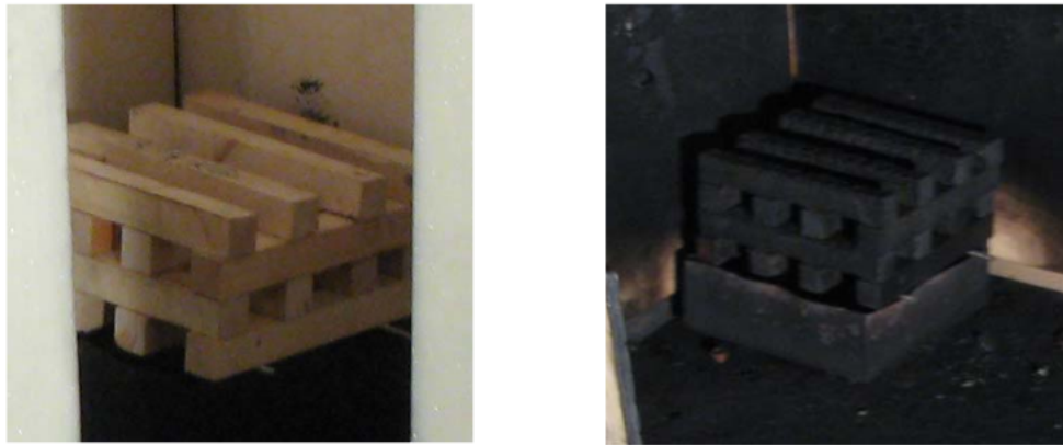
Figure 2. A wood crib before a fire experiment (left) and after the fire the experiment (right). The fire was extinguished with water before the crib had been completely consumed. The wood sticks had a cross-section of 40 mm x 40 mm and a length of 305 mm.
